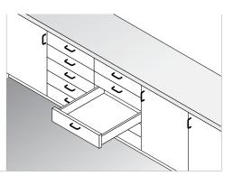
Identical mounting positions for Dynamic NT Full Access and Full Extension slide-on mounting.
